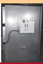
Your unit will ship complete with minimal assembly. Booths are constructed from 14ga steel, satin coat for long durability.
