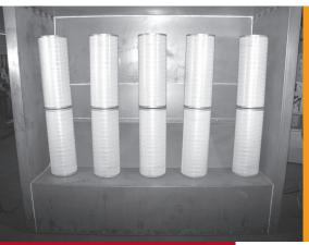
Cartridge filters designed to be above floor level to eliminate operator from pushing reclaim powder into cartridge filter. This extends the life of the cartridge and prevents clogging.
