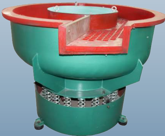
CL- AB type: spiral curved mouth with automatic separation sieve
